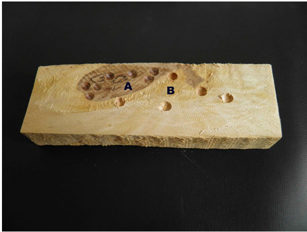
Fig. 1 Cylindrical block cut from the transverse section of birch ( Betula pendula ) log. A central, brownish ring; B peripheral, yellowish ring. Hollows in the wood indicate sites of sampling with the drilling device (according to Mackiewicz et al. 2019)
