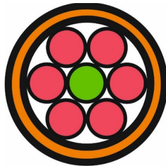
Figure 4. Scheme of a 1-to-7 fan-out fibre-optic bundle in a round-end configuration. The central core of the fan-out (green colour) transfers a back-reflected signal form the measuring head to the photodetector, while other cores (red colour) illuminate the tested sample.
